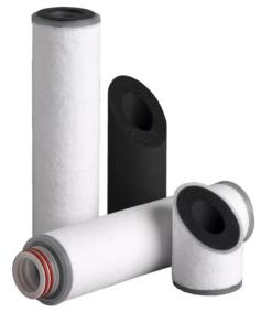
The **SupaCarb CP** carbon block uses a unique sintering process that combines both granular and powdered activated carbon. This results in the highest available surface area for adsorption of contaminants. The carbon block is protected by a spun-bonded, pure polypropylene fibre prefiltration layer, to produce a unique high performance module, offering superior on-stream life.
